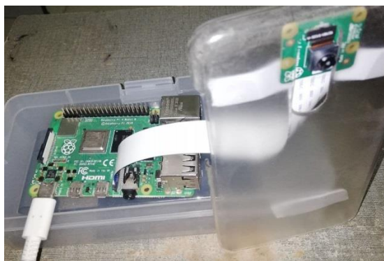
Figure 4: Shows the raspberry pi and the camera pi are connected with each other.
